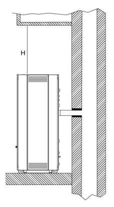
Minimum mandatory distance from flammable material and from roof for maintenance **H= 800 mm**
