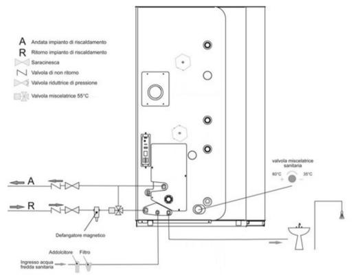
**Caution**: to prevent the heating system from having to be regularly cleaned it is best to **install a magnetic sludge remover**, this filter aids routine maintenance, increases boiler life span, aid removal of impurities and increased global efficiency of the system.
