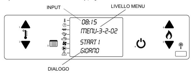
After having putting the first parameter (M-3-2-01) "DAILY CHRONO" to "on", you can set two startups and two shutdowns. For each parameter, you can set the startup or shutdown time or the value "off", if you do not wish to activate the daily programming.
